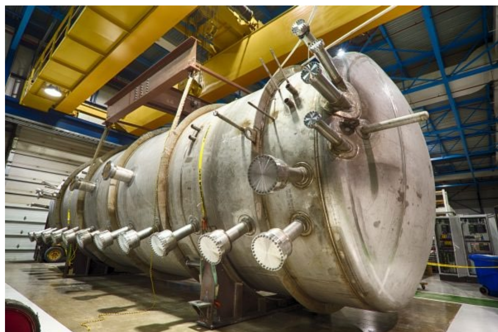
Images of the MicroBooNE LArTPC Detector. Image of the cryostat (left) and CAD diagram (right). Copied from microboone.fnal.gov/images-videos/
